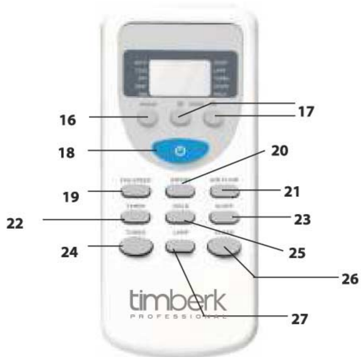
Figure 3. Description of the remote control board
